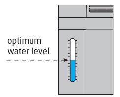
With the correct water level and the water cooling fans operating 24/7, the MAX water temperature will rise approx 4°C above room temperature
